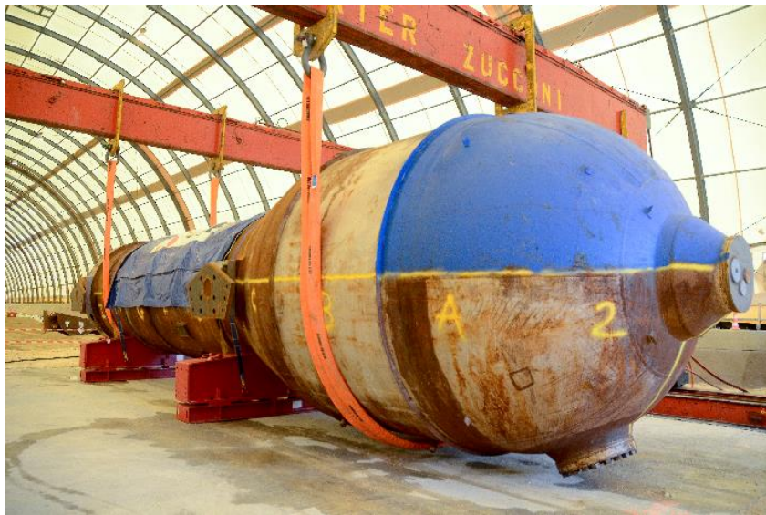
Figure 8: Disposal of a steam generator at Cires - Photo credit: Andra.
